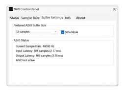
The Buffer Settings page allows you to view and set the buffer size of the current device's ASIO driver. You can select the desired buffer size from the drop-down menu. A smaller buffer size reduces audio latency to the host software, with buffers of 256 samples or less resulting in nearly imperceptible latency.
