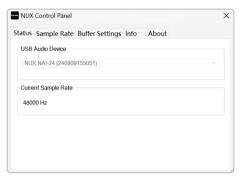
The Status tab shows the ID number of the USB audio device along with the current sample rate of the device.
